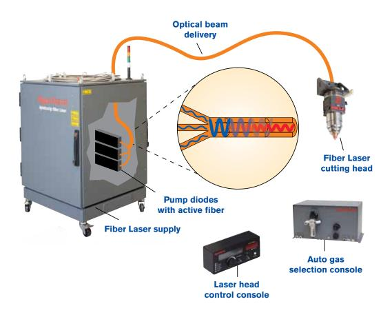
Multiple solid state pump diodes are combined to generate the laser beam which is then transmitted through a flexible delivery fiber to the laser cutting head.
